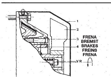
Its unique characteristic lies in its ability to exploit the motor flux and the brake shoe. This is due to the particular way in which the motor has been constructed, which allows the ferromagnetic insert to move towards the brake shoe anchor, which in turn is attached to the rotor when the motor is connected. When the motor is disconnected the rotor is blocked.
